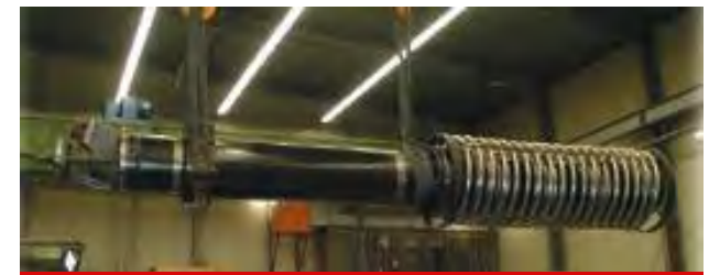
Submersible Motor for Cavern Pump
